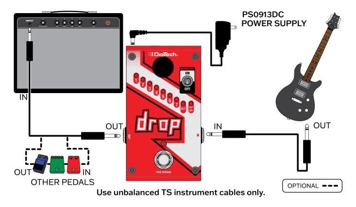
**NOTE:** The Drop should be the first pedal in your effects chain. Placing any effect in front of it can impact the pitch shifting performance.
