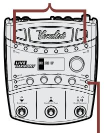
Make sure the settings match your system: Stereo/Mono Phantom Power Guitar XLR Level Guitar Sensitivity
