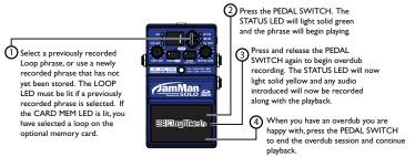
You can continue adding overdubs by continuing to press the **PEDAL SWITCH**. Each time an overdub is added, the last overdub is merged with the original loop and it can no longer be undone using the Undo feature. Once you are finished with overdubbing, press the **PEDAL SWITCH** two times quickly to stop playback/overdubbing.
