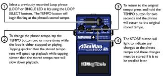
Press the **STORE** button twice to store Tempo changes if desired. You can play along with the adjusted playback speed and still be in tune since the pitch does not change based on playback speed.
