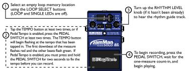
To set up a memory location with a tempo but not record to it, follow steps I and 2 and then store the new tempo using the Store procedure. When you return to the empty loop location, the tempo will already be set as indicated by the Tempo button flashing.
