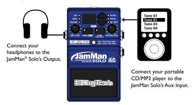
**NOTE:** All audio signals connected to the Aux input are summed to mono.
